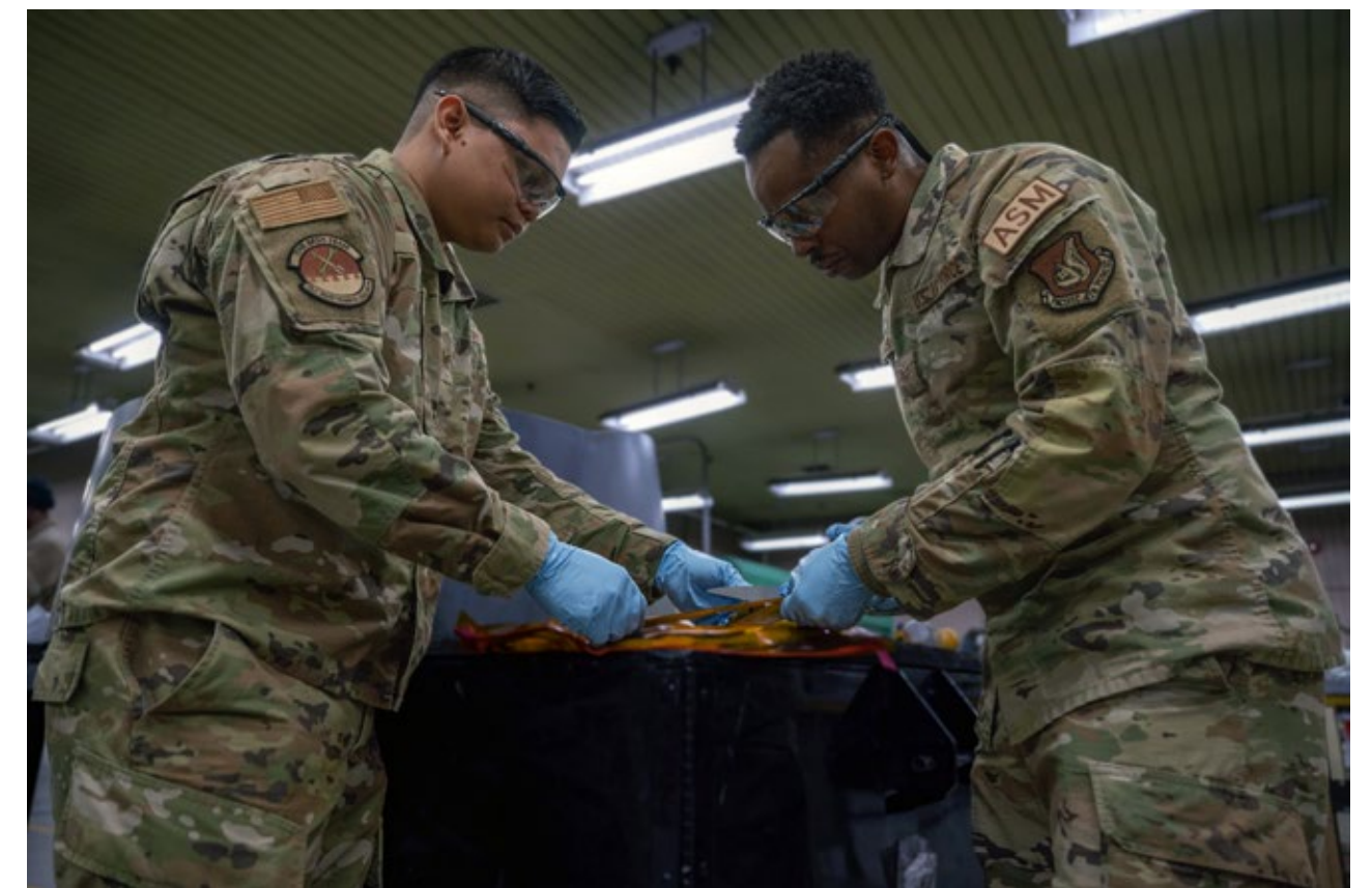
U.S. Air Force Staff Sgt. Sean Soriano, left, and Staff Sgt. Alan Roseman, 51st Maintenance Squadron aircraft structural maintenance craftsmen, trim a porous separator film at Osan Air Base, Republic of Korea, Feb. 8, 2024. This material is used in conjunction with resin and fiberglass to help create new aircraft structures. The 51st MXS follows tedious guidelines to optimize the functionality of the aircraft. (U.S. Air Force photo by Senior Airman Brittany Russell) ▲
