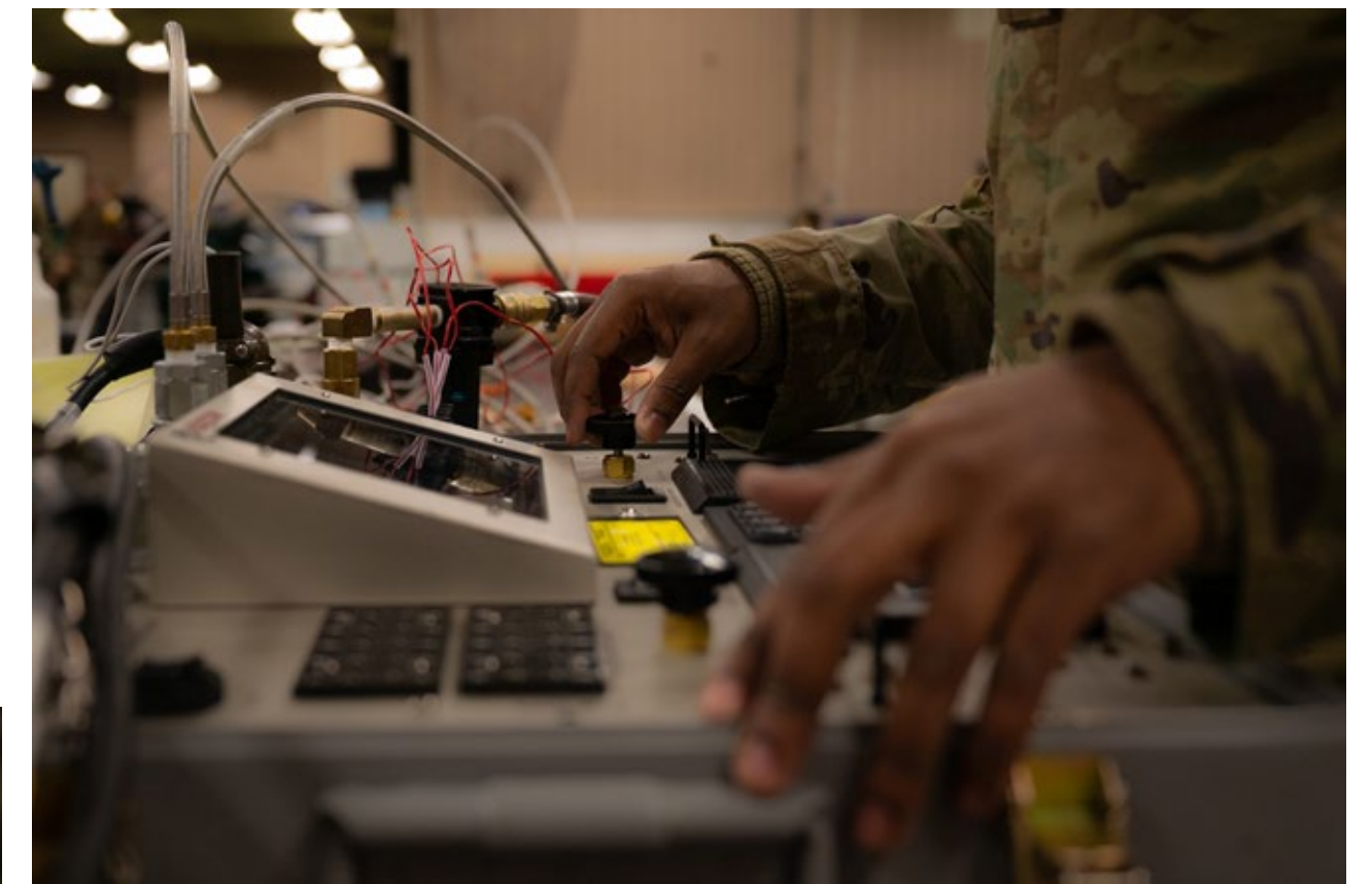
U.S. Air Force Staff Sgt. Alan Roseman, 51st Maintenance Squadron aircraft structural maintenance craftsman, prepares a hot bonder at Osan Air Base, Republic of Korea, Feb. 8, 2024. A primary function of the hot bonder is to create a vacuum seal and regulate pressure. The 51st MXS utilizes technology that ultimately optimizes the performance of the 51st Fighter Wing aircraft. (U.S. Air Force photo by Senior Airman Brittany Russell) ▲
