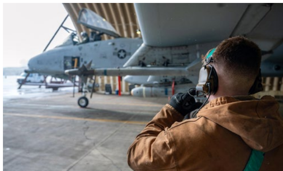
U.S. Air Force Airman 1st Class Tucker Arnold, 25th Fighter Generation Squadron crew chief, communicates with a pilot during a pre-flight systems check at Osan Air Base, Republic of Korea, Jan. 22, 2024. Airframe, powerplant and general Airmen are responsible for final pre-flight inspections to prevent the aircraft from being flown with malfunctions or hazards. (U.S. Air Force photo by Airman 1st Class Chase Verzaal) ◀
