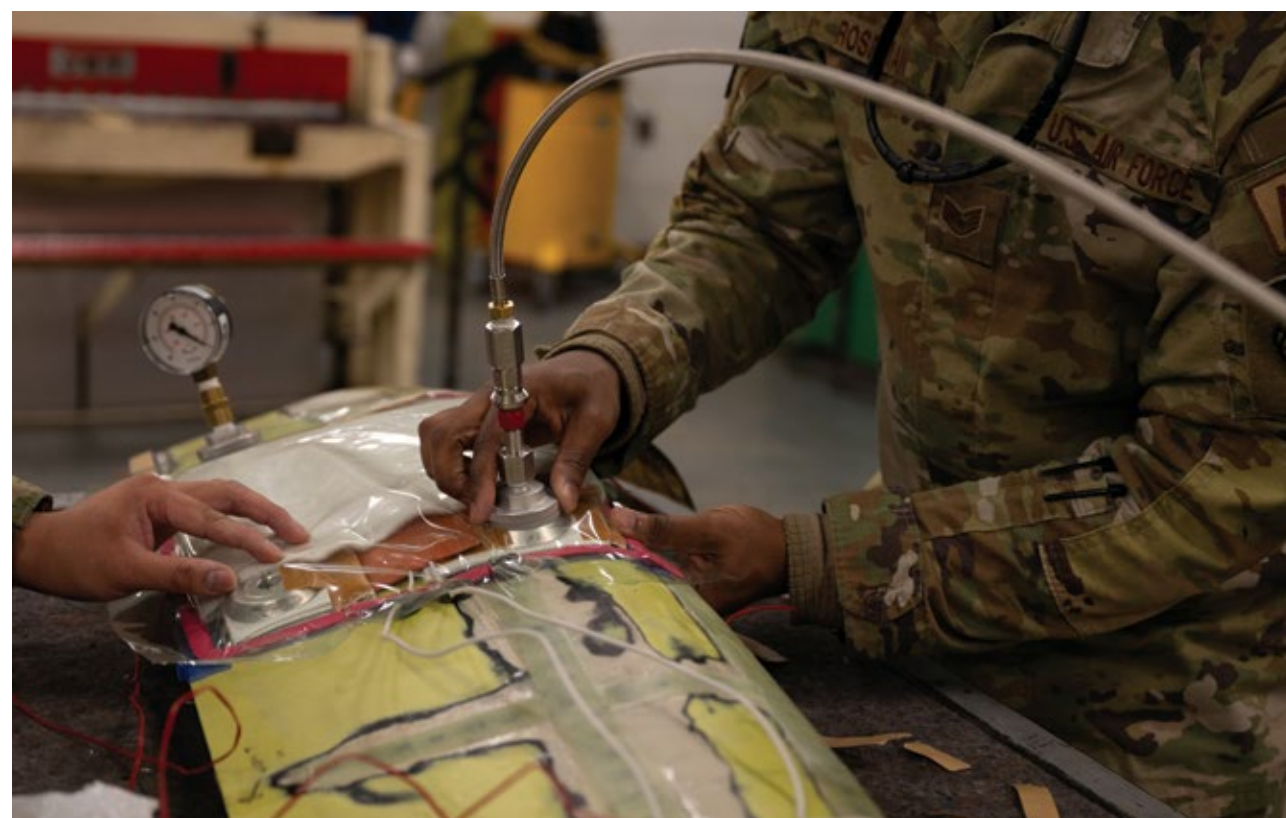
U.S. Air Force Staff Sgt. Alan Roseman, 51st Maintenance Squadron aircraft structural maintenance craftsman, prepares a vacuum seal hose at Osan Air Base, Republic of Korea, Feb. 8, 2024. The pressure going through the hose is regulated to ensure a smooth, seamless seal of fiberglass laid on the structure. Precision in structural aircraft maintenance is paramount to guaranteeing peak performance of 51st Fighter Wing aircraft. (U.S. Air Force photo by Senior Airman Brittany Russell) ▲
