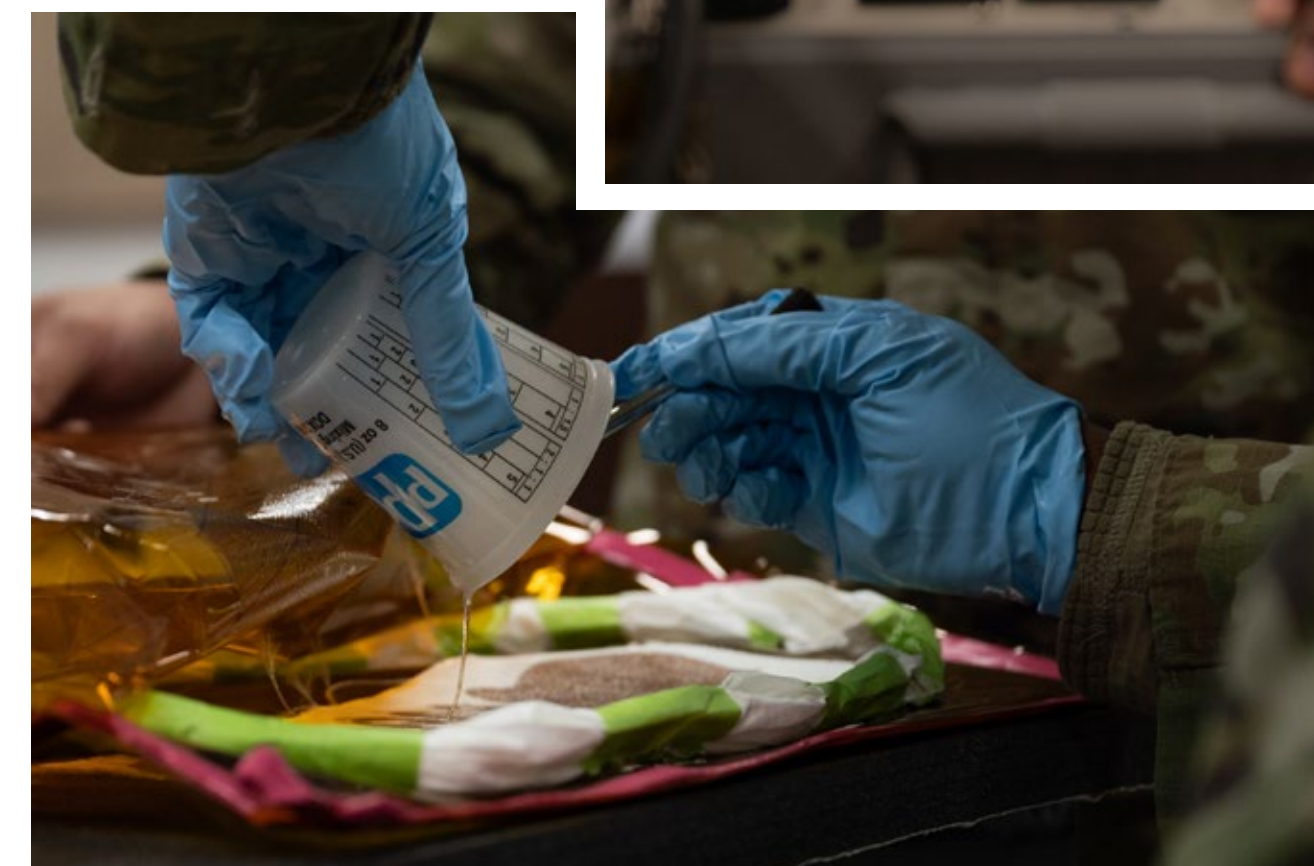
U.S. Air Force Staff Sgt. Alan Roseman, 51st Maintenance Squadron aircraft structural maintenance craftsman, prepares a hot bonder at Osan Air Base, Republic of Korea, Feb. 8, 2024. A primary function of the hot bonder is to create a vacuum seal and regulate pressure. The 51st MXS utilizes technology that ultimately optimizes the performance of the 51st Fighter Wing aircraft. (U.S. Air Force photo by Senior Airman Brittany Russell) ▲
